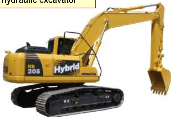
HB205 hybrid hydraulic excavator
