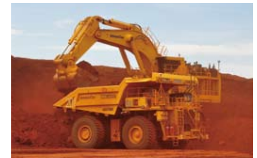
930E driverless dump truck in an iron ore mine in Australia
