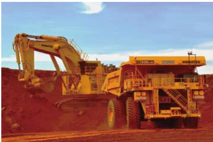
Driverless 930E dump truck in operation at an iron ore mine in Australia
