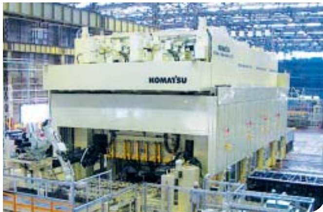
▲ Komatsu has received Toyota Motor's Technology & Development Award for this AC Servo motor-driven large press.
