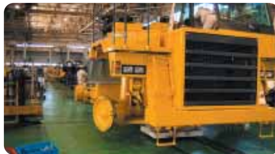
Assembly line for dump trucks at Komatsu (Changzhou) Construction Machinery
