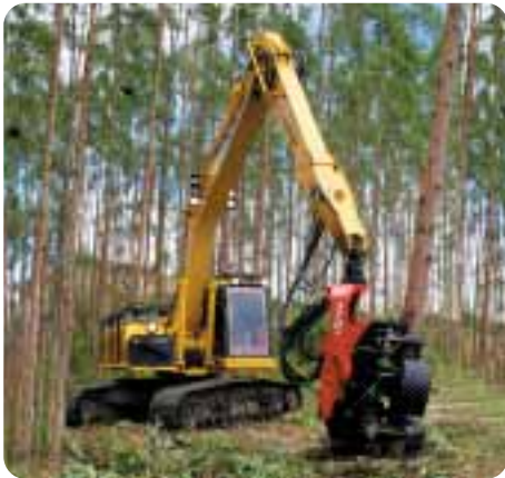
Komatsu Forest-made Valmet 370E harvester head attached to Komatsu's PC200 hydraulic excavator
