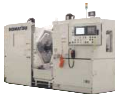
Crankshaft miller made by Komatsu Machinery Corporation
