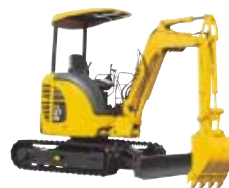
PC27MR-2 mini hydraulic excavator with tight tail swing launched in March 2004
