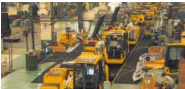
Assembly lines for hydraulic excavators at Komatsu Shantui Construction Machinery
