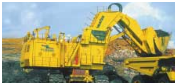
PC8000 super-large hydraulic excavator produced by Komatsu Mining Germany GmbH and delivered to iron-ore and other mines around the world, including the Central and South Americas
