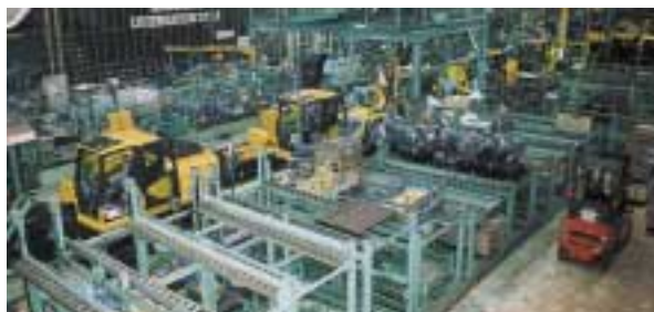
Assembly line for hydraulic excavators at the Osaka Plant operating at a high rate
