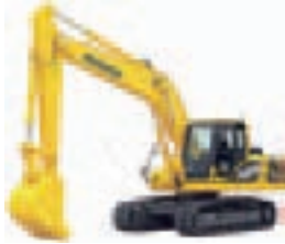
HB205-1 hybrid hydraulic excavator
