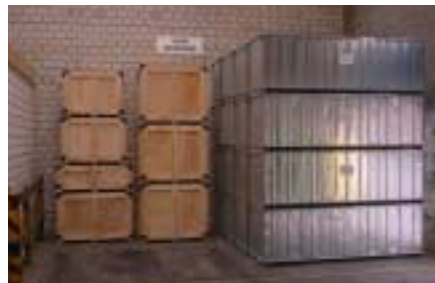
Improving packaging: conventional product-specific wooden crates (left) General-purpose steel boxes made to fit into containers (right)
