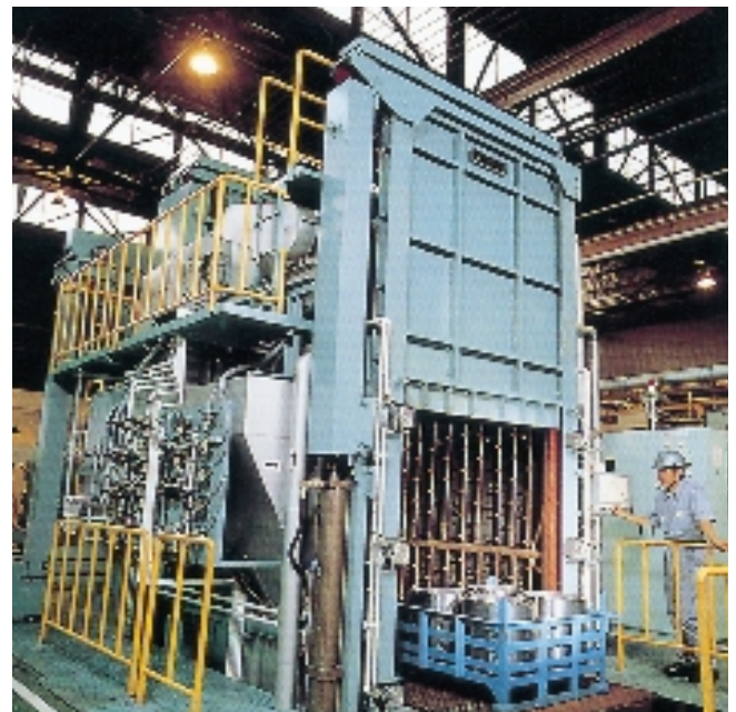
Gear-cleaning Unit at the Osaka Plant (Washing: water-based alkaline cleaner)
