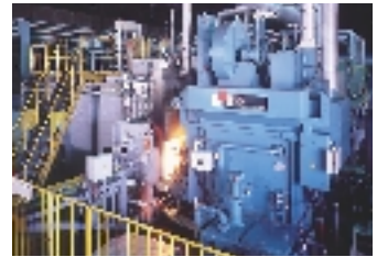
Rotary Hearth-type Flexible Carburizing Furnace
