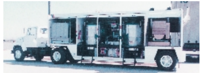
Trailer-loaded distillation equipment
